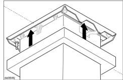
■ Finally, being careful not to scratch the chimney, push the cover plate up until the spring fixing clips click into place. If installed correctly, the cover should be secure and flush against the ceiling.
